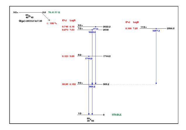
Figure 11. Zirconium-89 decay scheme<sup>16</sup>
