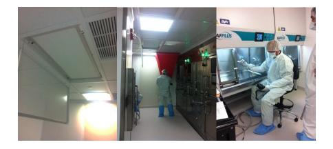
Figure 13. Images of ISO 7 GMP area certification process (left) HEPA filer in the ceiling, (middle) HEPA filter leak test, (right) ISO5 smoke test
