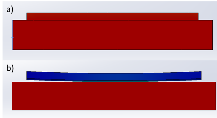
Figure 7 Side view of substrate on platen. a) Represents typical substrate prior to print with no warping. b) Represents typical warping of substrate experienced during a LENS 3D print. Platen in red and substrate in blue.
