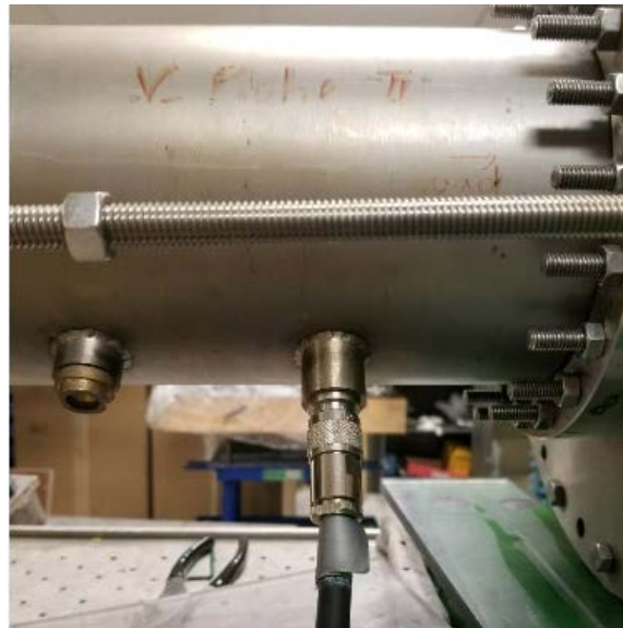
Figure 4-10: Photograph of the D-dot sensor input on outer conductor of coaxial transmission line.
