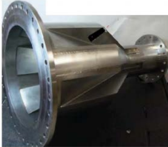
Figure 1-1: Photograph of the Magnetron with Diffraction Output (MDO).
