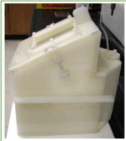
Figure 21: Side view of custom built electroplating bath reservoir showing graded lid, process viewing window and backside location for fluid input, output, thermocouple and heaters.
