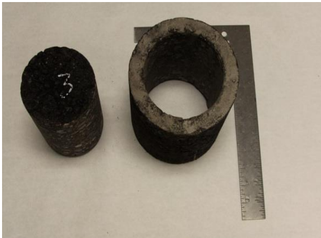
Figure 3.6 100mm specimen cored out of a 150mm compacted specimen.
