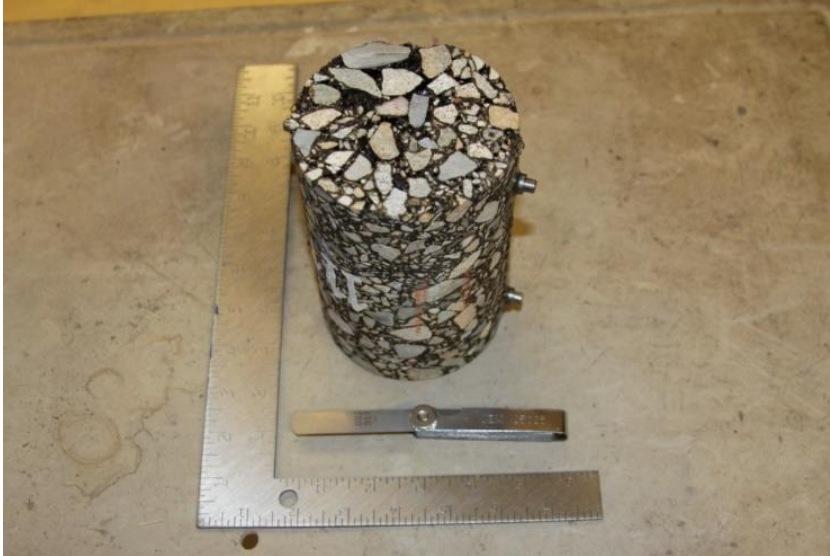
Figure 3.9 Straight edge and feeler gauge for Waviness check.
