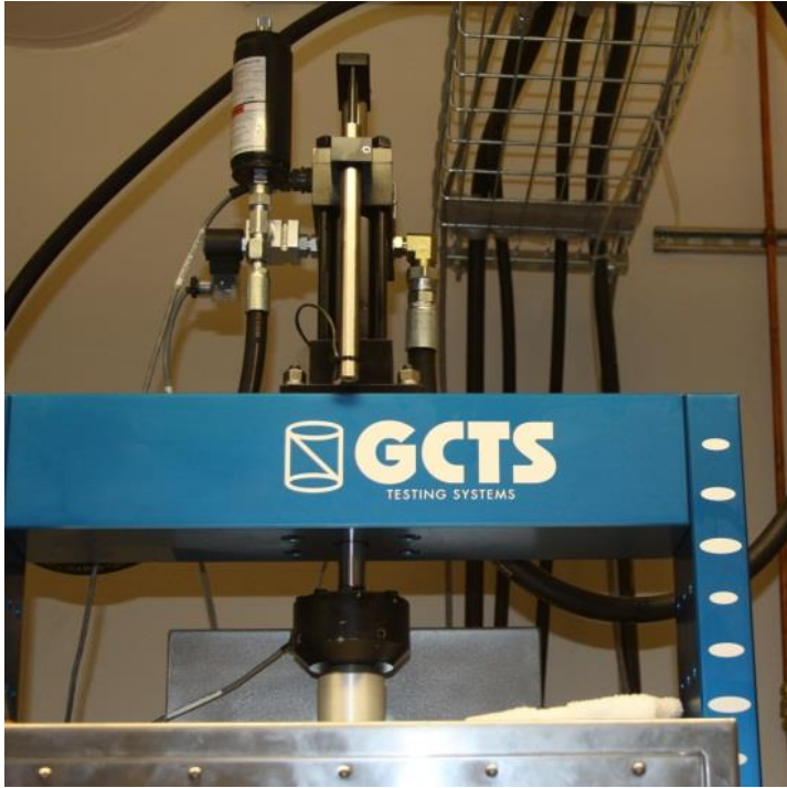
Figure 3.15 25kN Load Cell Connected to a 25 kN Actuator.
