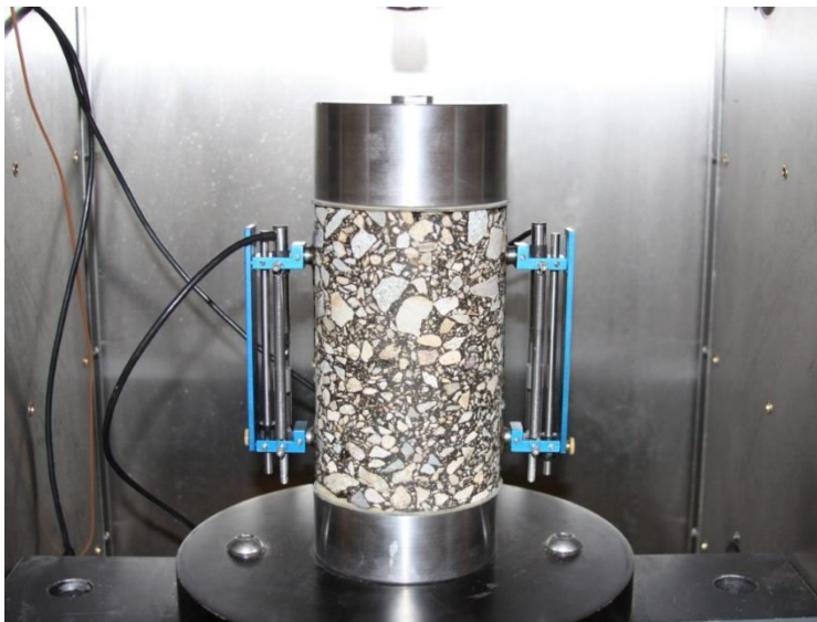
Figure 3.16 Linear variable differential transformers (LVDTs) mounted on specimen.
