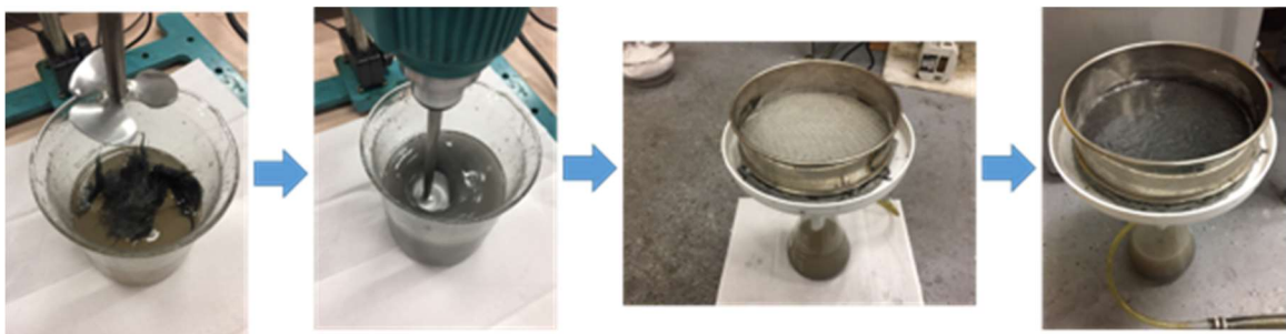
Figure 17 Non-aligned mat production process involving dispersion of recycled fibers into viscous glycerol solution and deposition of fibers onto nylon covered sieve.
