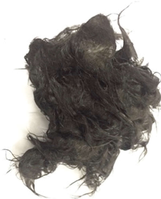
Figure 3 As received recycled carbon fibers from Adherent Technologies, Inc.
