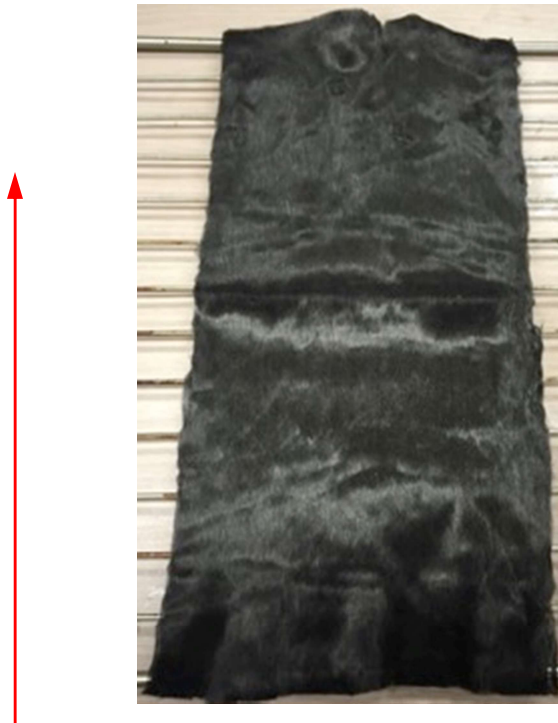
Figure 19. 1.5g mat of aligned recycled carbon fibers, approximately 5"x10". The red arrow shows the fiber alignment direction.
