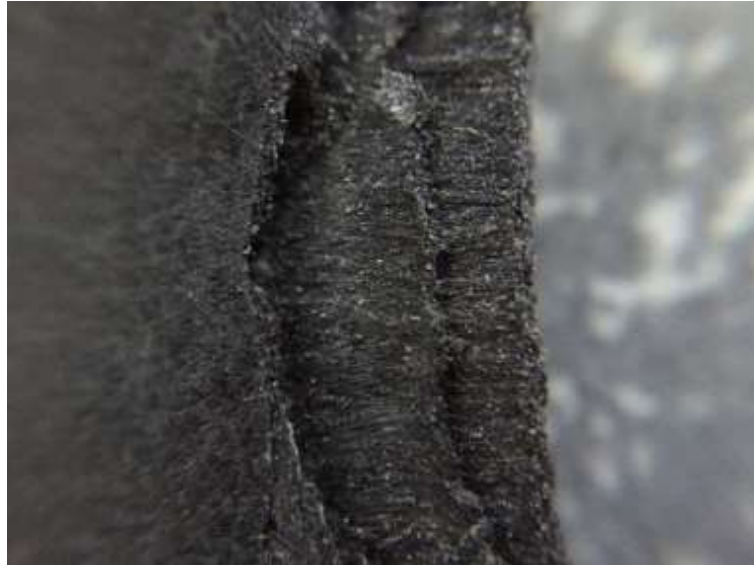
Figure 31 Fracture surface of carbon fiber composite specimen
