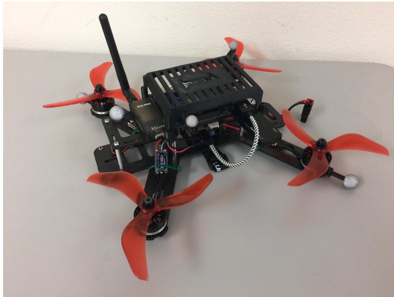
Figure 2.3: QAV250 frame based quadrotor with Odroid XU4 microprocessor on top of it and Vicon markers attached. The Odroid is secured by a custom design and 3D printed part.
