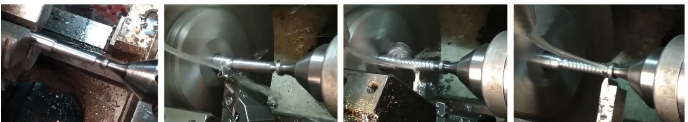
Figure 16 - Turning process: profile roughing, profile finishing, thread roughing and thread finishing
