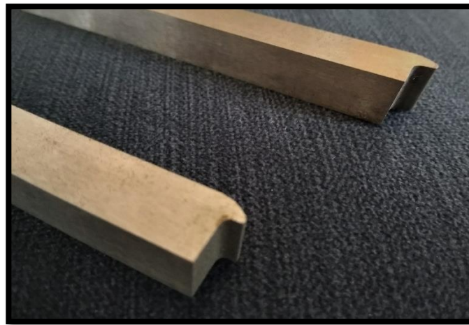
Figure 17 - Custom made HSS-Co threading tools
