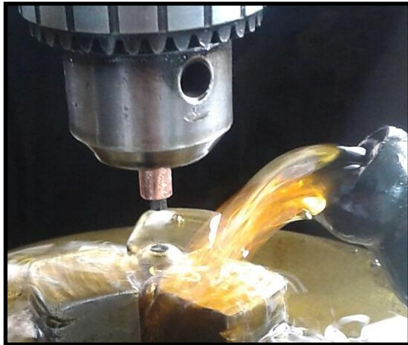
Figure 18 - Hexagonal socket EDM by penetration
