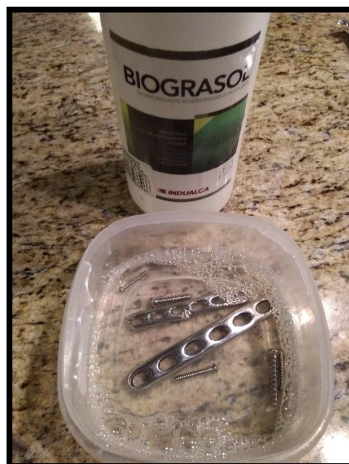
Figure 25 - Pre-passivation cleaning process
