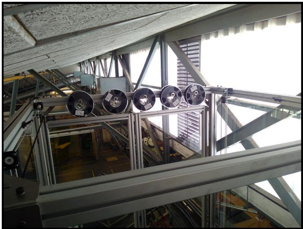
Figure 4.20: Top View of Printer – Printing Material Reel System
