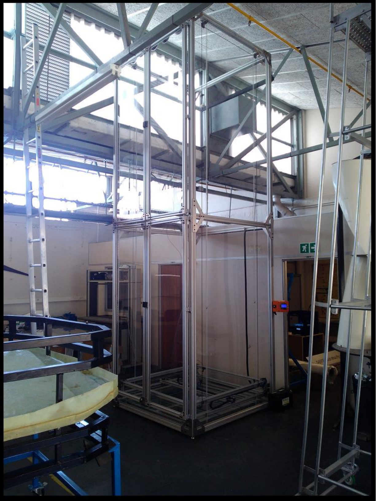
Figure 4.21: Full Isometric View of Large-Scale Additive Manufacturing Platform
