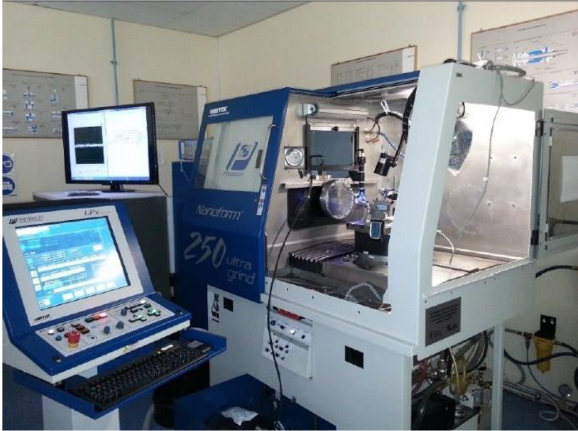
Figure 3.3: Nanoform® 250 ultra-grind Precision Diamond Turning Lath at Precision Engineering Laboratory, Nelson Mandela Metropolitan University
