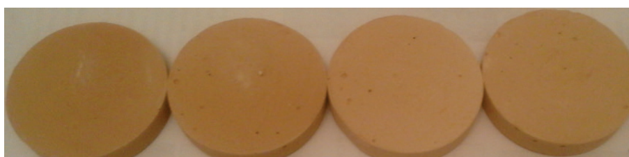
Fig.3-Cooking temperature of Bouhanifia’s mud (900°C, 950°C, 1000°C and 1050°C)
