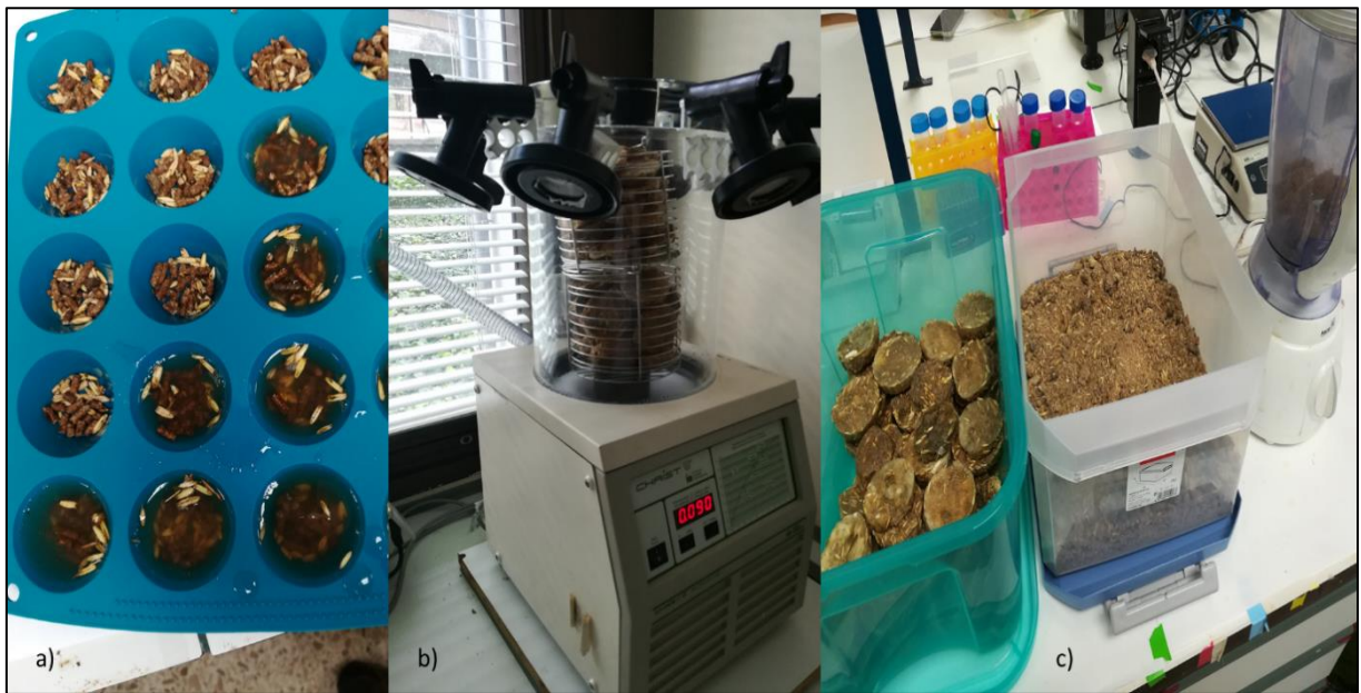
Figure 9 - Product manufacture steps (original): a) Pouring gelatine mixture into silicone moulds. b) Lyophilization machine. c) Product mashing in a blender.
