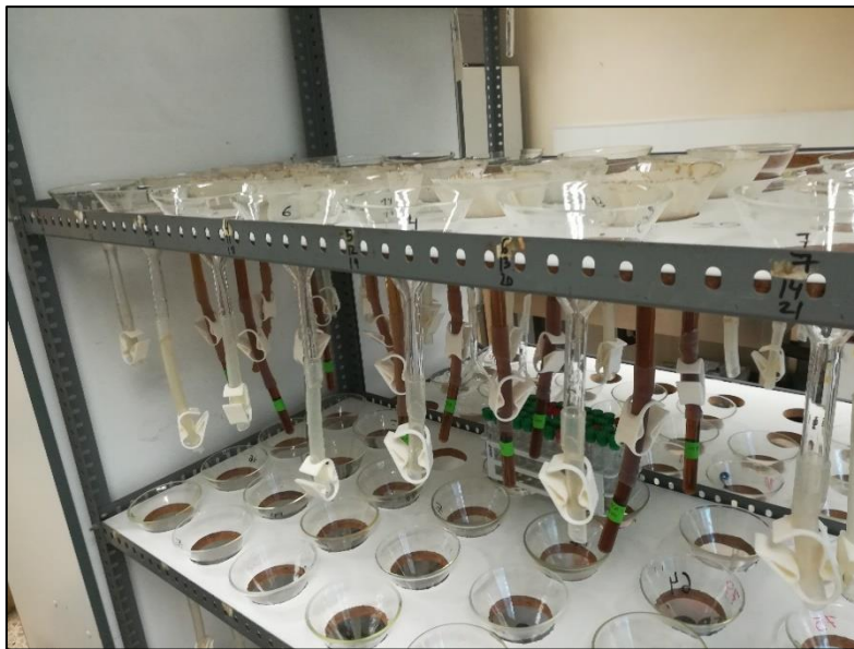
Figure 17 - Assembled Baermann apparatus for the retrieval of larvae (original).
