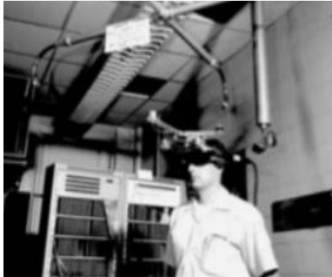
Figura 13 - Ivan Sutherland com o “Head Mounted Three Dimensional Display” (Negroponte, 1970)
