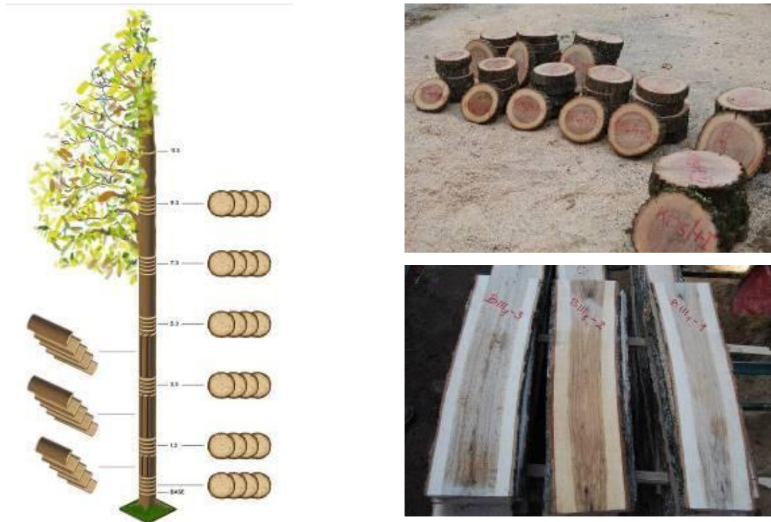
Figure 3.9., 3.10. & 3.11. General sampling plan of the felled trees and aspect of the disks and boards
