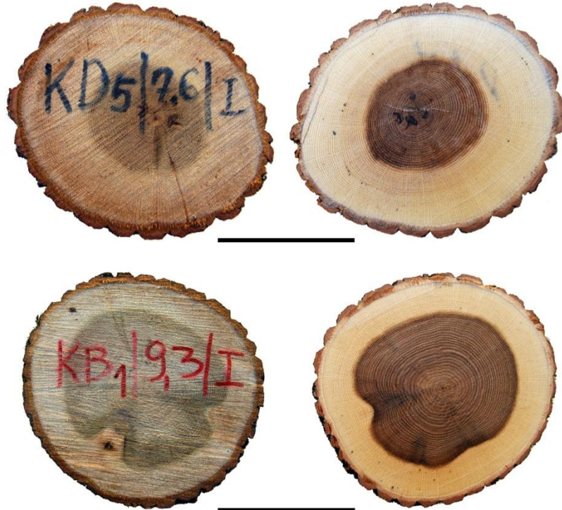
Figure 2.10. Cross sectional discs of Quercus cerris from Duboçak (KD) and Blinaja (BB), Kosovo, showing heartwood and sapwood colour differences
