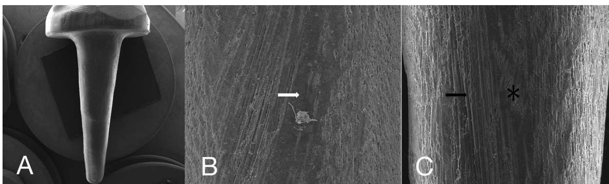
Fig. 4: SEM micrograph of the customized CAD/CAM glass fiber post and core design (A), and of the surface characteristics after ethanol application (B) or hydrogen peroxide (C). The white arrows show the epoxy layer covering the fibers and the black arrows show the exposed glass fibers. Asterisks shows the areas where damage to fiber integrity has occurred, caused by the CAD/CAM milling procedure.
