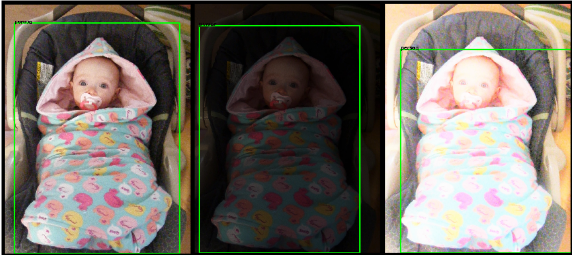
Figure 4.7: YOLO image brightness variation confidence, left to right - 0.71; 0,77; 0.47
