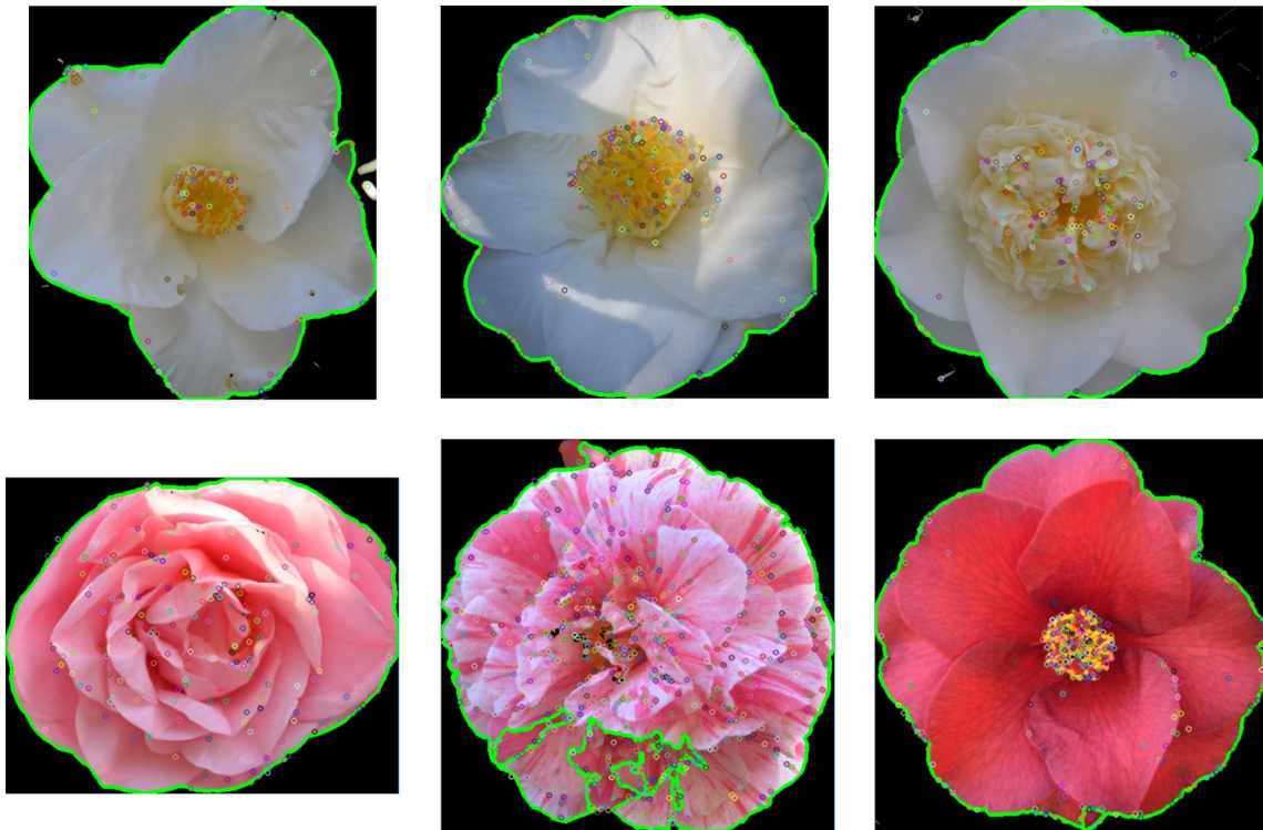
Figure 3.17: Examples of SIFT key points. The green region indicates where the SIFT key points must be extracted from. The points indicate the extracted SIFT key points.
