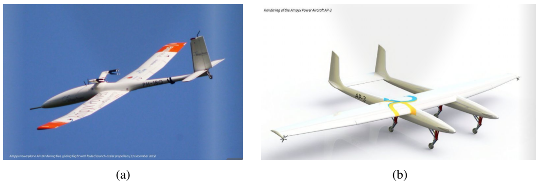
Figure 2.7: Ampyx Power prototypes. (a) AP-2 20kW prototype during a free gliding flight; (b) Rendering of the AP-3 aircraft [20].
