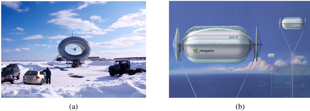
Figure 2.11: Lighter than air systems. (a) Altaeros prototype [24]; (b) Magenn Power concept [25].
