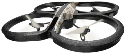
Figure 1.1: Parrot AR Drone 2.0 quadrotor is controlled by a smartphone.
