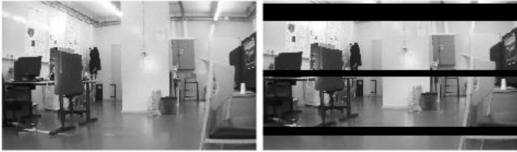
Figure 5.15: Snapshot of the video stream at the sink. With CSMA/CA (on the right), relays cannot handle every received packet, dropping some that appear as black lines in the image. Under DVSP (on the left), video streaming is visibly improved and frames are generally complete.
