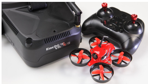
Figure 1.3: Eachine E013 is a low-cost micro quadrotor equipped with camera and FPV headset.
