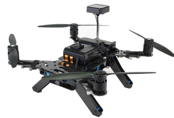
Figure 1.4: Intel Aero research platform comes with a vast set of external sensors.
