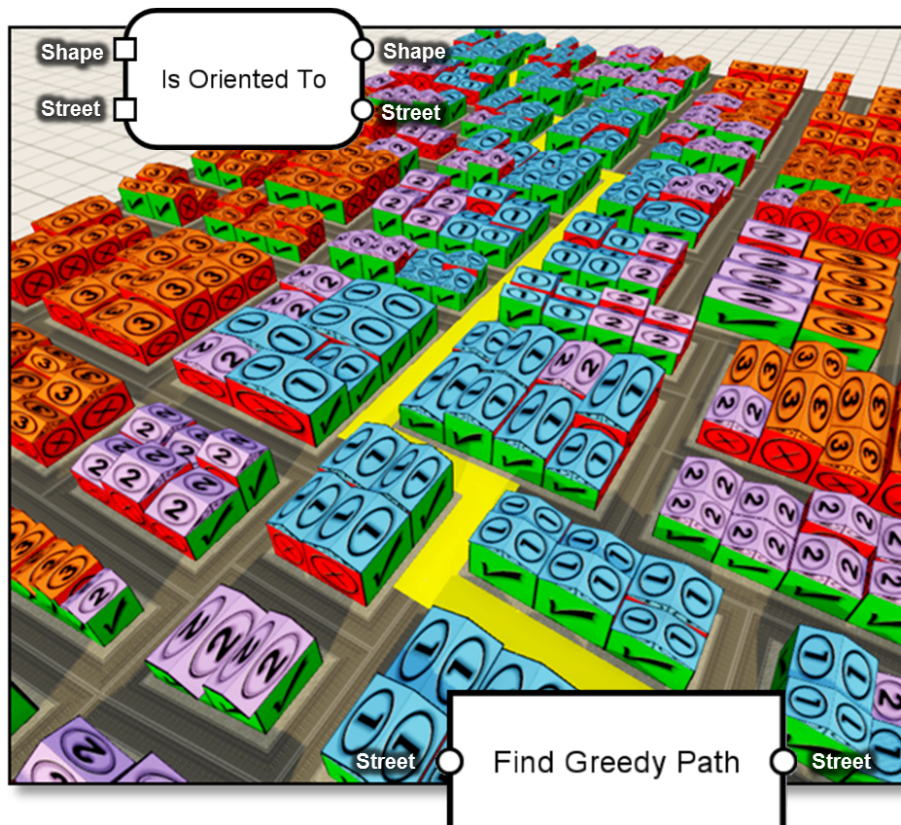
Figure 4.4: This approach introduces context-awareness verifications which can be applied at any step of the generation process. Here, visibility calculations are performed to determine which facades are visible (marked in green) from a highlighted street (marked in yellow and black), and which are not (marked in red). The minimum distance of each house towards that same street is calculated, and the decision on the level of detail (1, 2 or 3, as marked on the roofs) is based on the distance. For applications focused on a main path (such as racing games), this information could be used to guide the procedural content generation and include budget considerations in the level construction.
