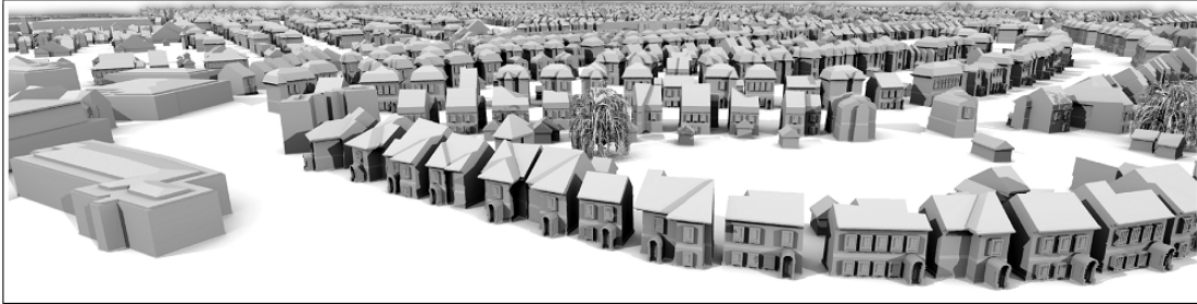
Figure 2.21: Procedural extrusion approach on building floorplans from GIS [KW11].
