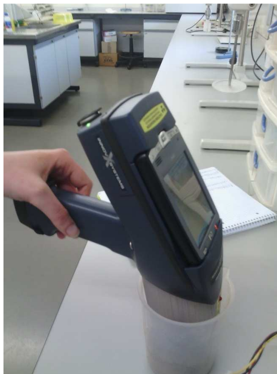
Figure 4.9 - Portable X-Ray Fluorescence Analyzer used to determine chemical composition
