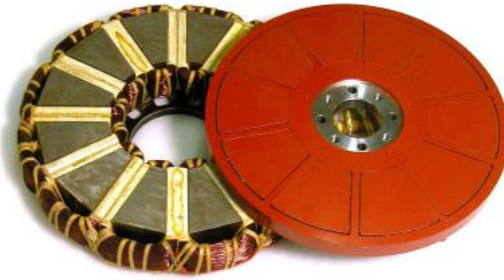
Figure 2.1- Pancake axial flux PMSM [6]
