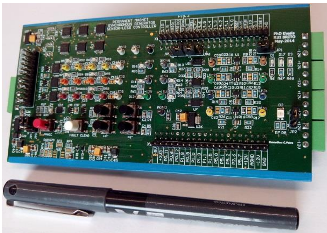
Figure 7.11- Controller interface Board - front side
