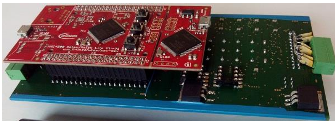
Figure 7.12 - Controller interface board - back side with piggybacked XMC4500 kit
