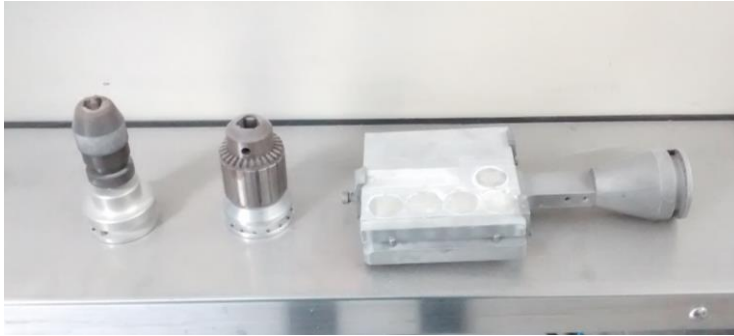
Figure 6.4 - Comco LA3250 Advanced Lathe part tooling. Two mandril pieces and a platform are provided to coat different piece geometries.
