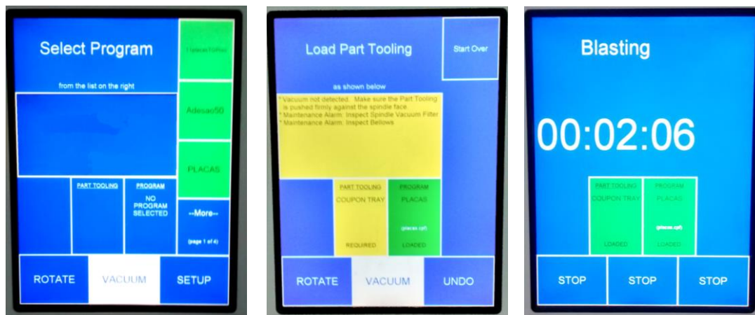
Figure 6.5 - Comco LA3250 Advanced Lathe user interface. The user can select the piece to coat on the right side of the pane (A), after selecting the coating program if the part tooling is not correctly detected or is not the correct part tooling for the program about to start an alert in yellow is displayed (B) when the problem is solve the user can start the coating program and the countdown starts (C).
