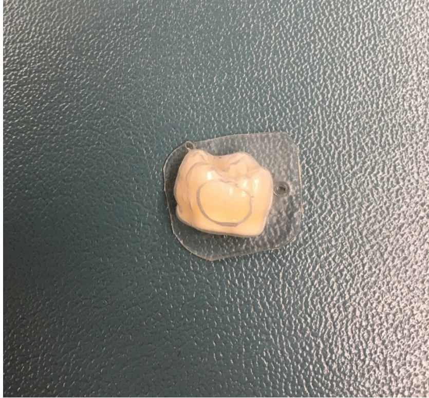
FIGURE 6. Crown sample mounted in the custom-made close-fit cap made by a clear soft thermoplastic sheet.
