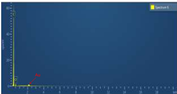
Figure 9. Typical EDS spectrum from a tar ball particle containing only C and O. (The gold peaks are artefacts that originate from the gold-coated membrane filters)
