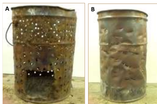
Figure 1: Illustration of imbaulas used in the experiment: (A) high ventilation case, (B) low ventilation case.
