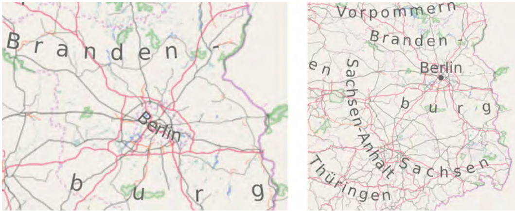
■ Figure 6 Labeling of an area using an area label (left) and a point label at smaller map scale (right) (© OpenStreetMap contributors).
