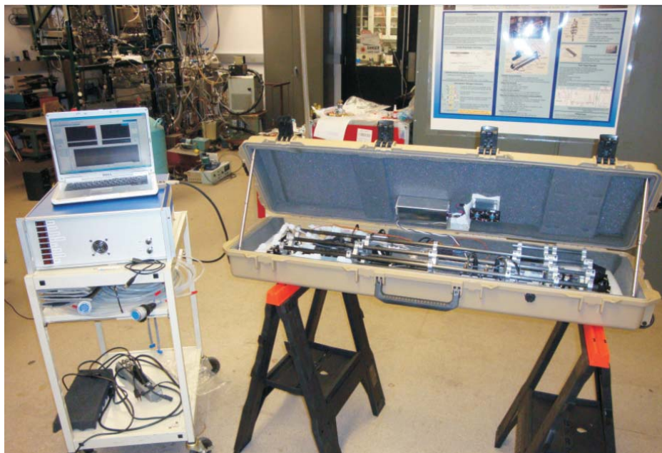
Figure 8-8: The earliest version of the new cage design that was employed in the NOxCaRD instrument in 2009.
