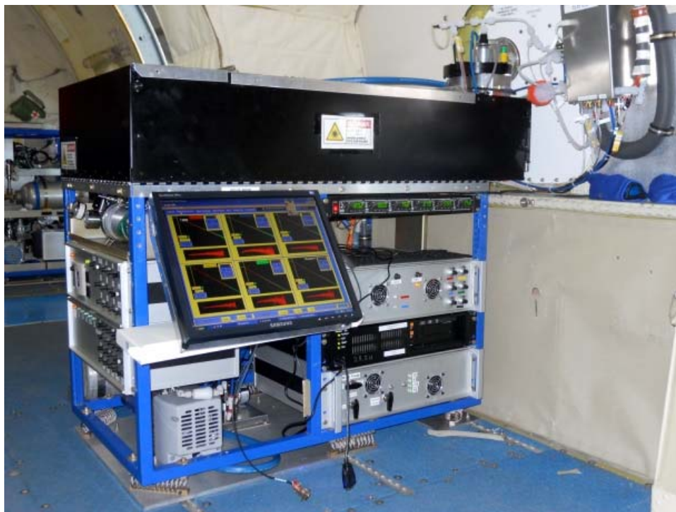
Figure 2-3: The current 6-channel ARNOLD instrument installed in NOAA P-3 research aircraft. Results from the corresponding campaign are outlined in Publication D (Chapter 6).
