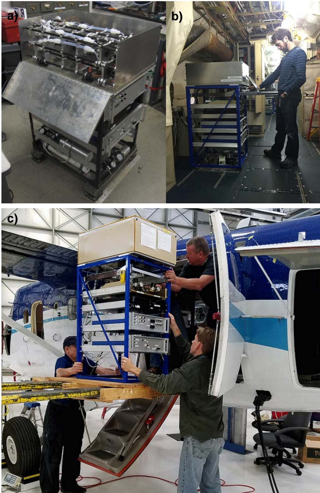
Figure 2-6: a) NOxCaRD instrument with 4 channels. b) NOxCaRD installed in the NOAA P-3 Hurricane Hunter airplane. c) NOxCaRD being loaded onto the NOAA Twin Otter airplane in 2017. Photo by C. Womark.
