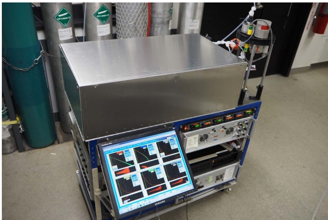
Figure 8-10: The intermediate version of the new ARNOLD instrument. The automated filter changer described in section 8.2 can be seen to the right in the picture.
