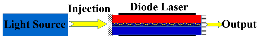
Figure 1.5: Schematic of semiconductor laser subject to optical-injection.
