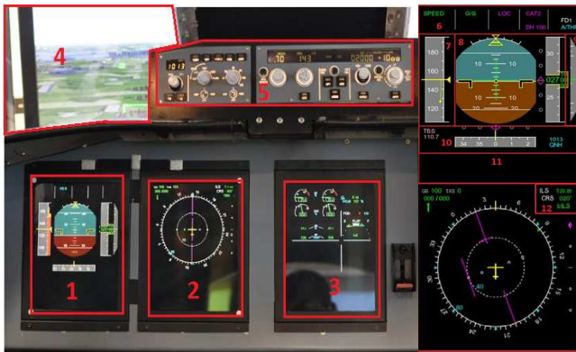
Figure 1: Cockpit Display with Areas Of Interest and Sub-AOIS: (1) Primary Flight Display (PFD), (2) Navigation Display (ND),(3) Electronic Centralized Aircraft Monitoring (ECAM), (4) Out of Window (OTW),(5) Flight Control Unit (FCU), (6) Flight Mode Annunciator (PFD.FMA) , (7) Speed Tape (PFD.SPD), (8) Attitude indicator (PFD.ATT), (9) Vertical Speed Tape (PFD.VS), (10) Heading Tape (PFD.HDG), (11) Message Zone (PFD.MSG), (12) Navigation display indicator of the PFD.
