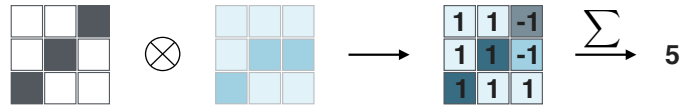
Figure 6.5.: A convolutional filter operates on a small section of the image that is of the same size as the filter itself. By a pixel-wise comparison of the filter and the image section and subsequent summation, a single value is obtained.
