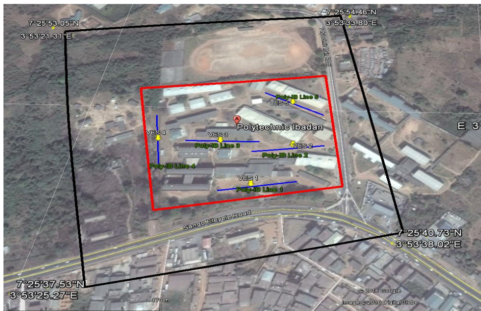
Fig. 2: Satellite imagery map of the study site in Ibadan indicating the 2D resistivity profile lines (blue) and VES points (yellow arrows)
