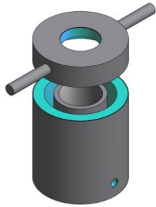
Figure 2: Exploded view showing part of furnace
