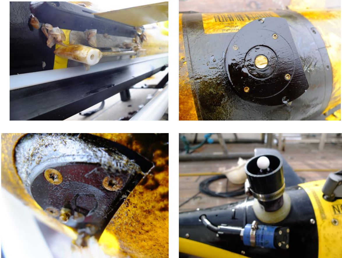
Figure 5: Photos of sensors on the summer deployed glider (unit 399) following recovery. The extent of biofouling on exterior components is clearly evident and resulted in critical degradation of data quality from optical sensors.
