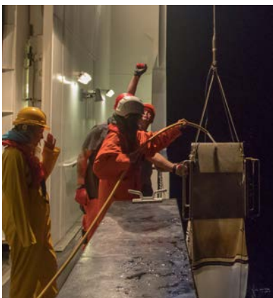
Multinet in continuous use in order to study plankton communities.
