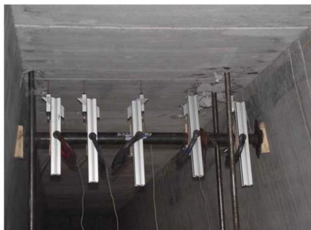
Figure 4. Position of the electronic displacement transducers.
