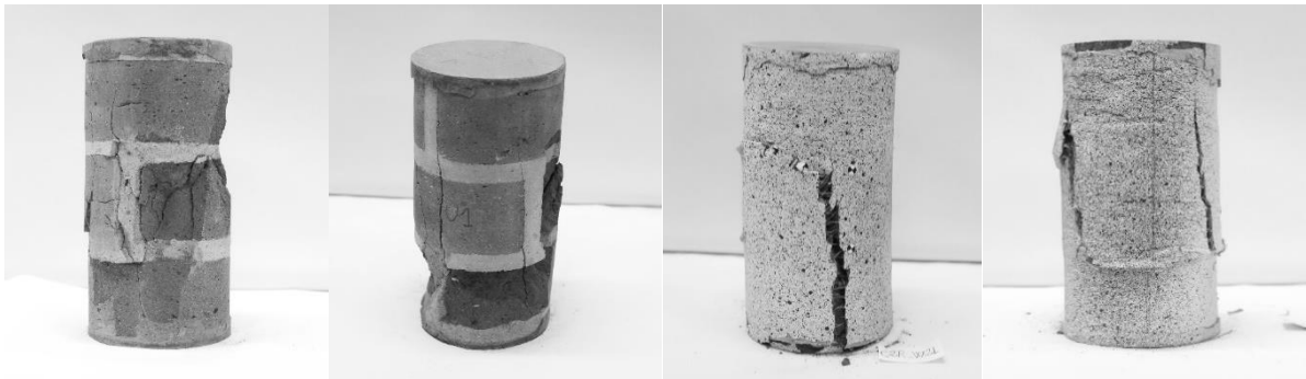
Figure 5: Photos of failed cylinders: a) unconfined (Scheme I); b) unconfined (Scheme II); c) Two layer BFRP grid wrapped (Scheme I); d) Two layer BFRP grid wrapped (Scheme II).
