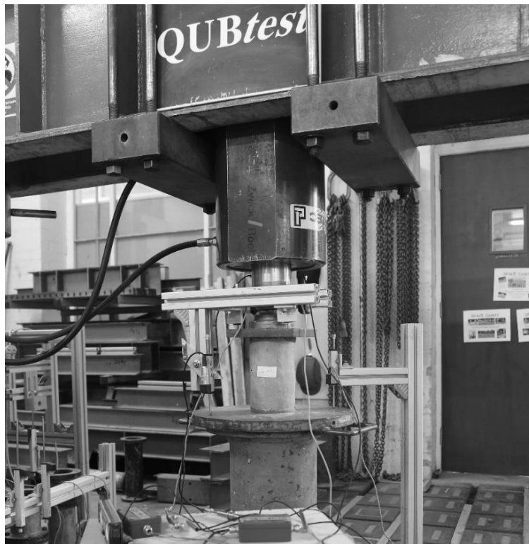
Figure 3: Photo of compressive test setup
