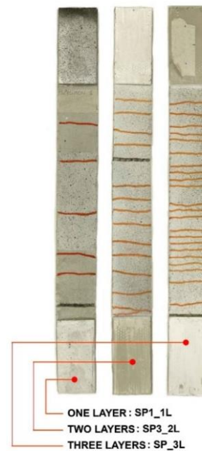
Figure 6. Crack pattern of composite specimens at failure.
