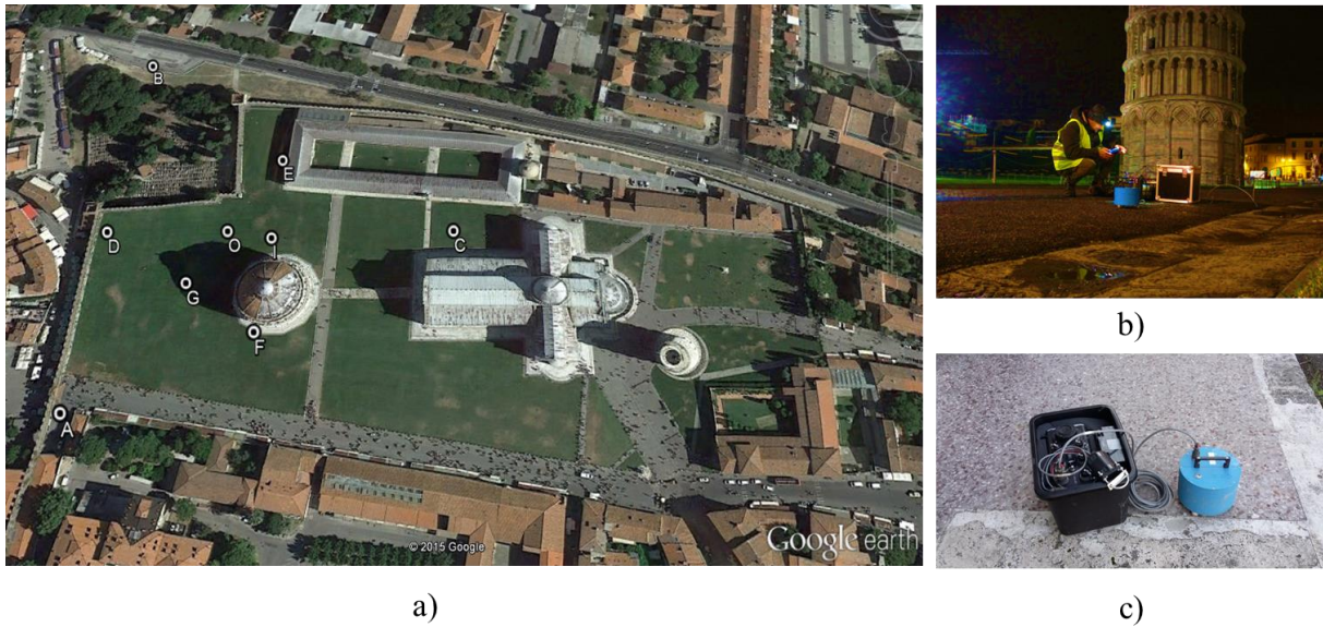
Figure 7. (a) Array2D test in Piazza del Duomo in Pisa: a) layout of the instruments in the square; (b) Installation of one the seismic stations; (c) Measurement station formed by REFTEK130 seismic stations and Lennartz 3D 5s velocimeters
