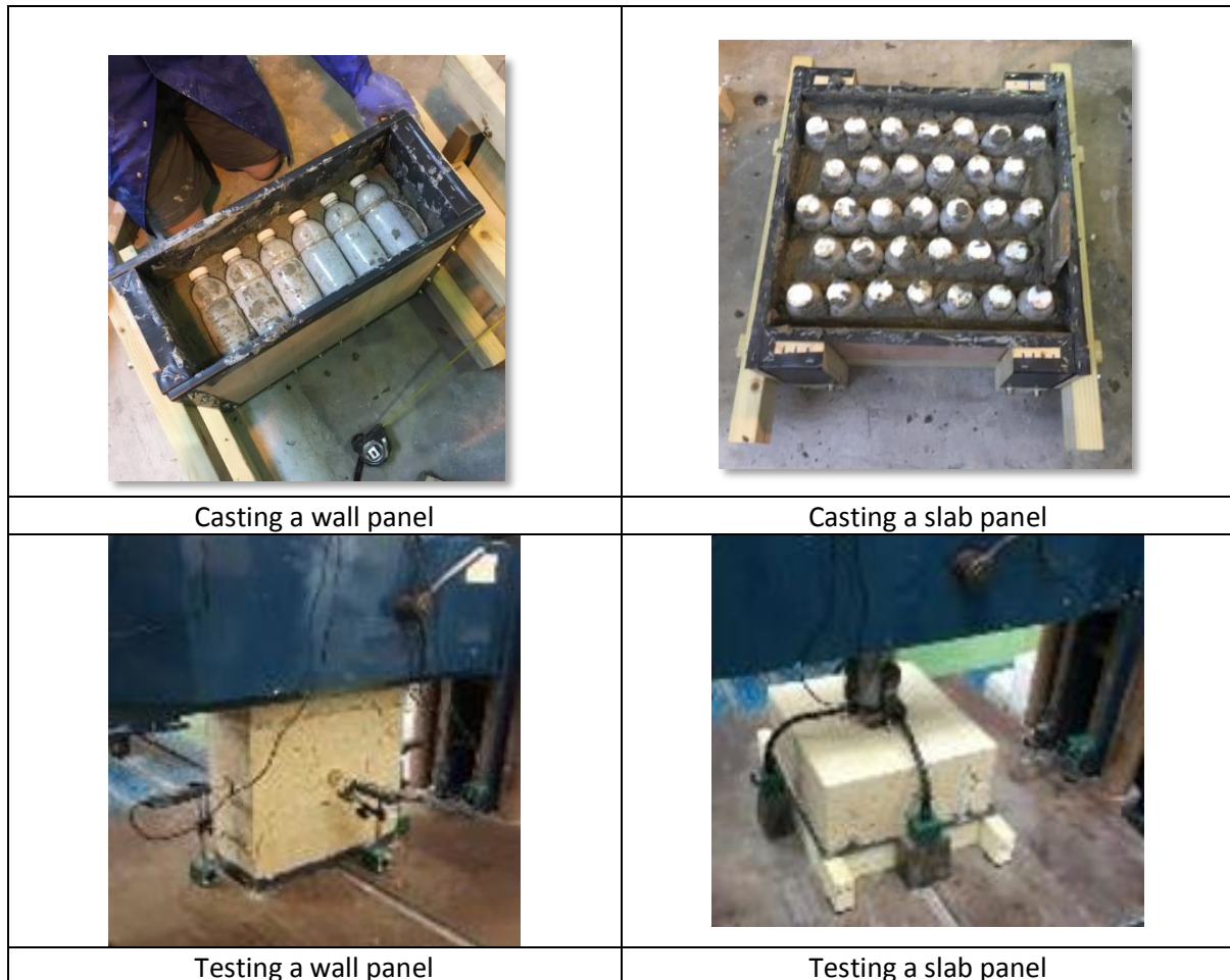
Figure 4: Casting and testing of wall and slab panels.
