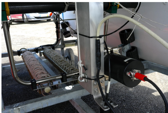
Figure 4. ULISSE configuration for the WiMUST system: the acoustic sparker and the two acoustic modem transducers can be seen in the middle part and front part respectively.
