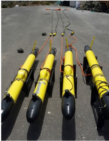
Figure 11. Folaga AUVs towing streamers with hydrophones.
