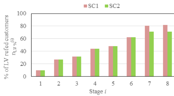
Figure 9. Percent of re-fed LV customers in SC1 and SC2, with respect to the total number of LV customers for each stage of the restoration plan.
