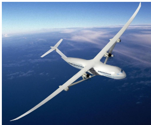
(b) Truss Braced Wings
