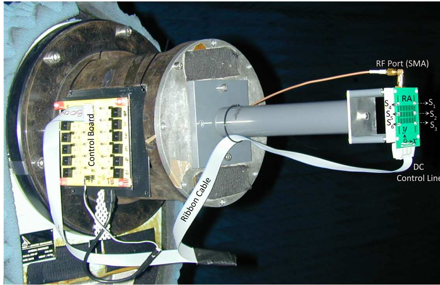
Fig. 5: Photograph of the RA measurement setup showing numbered inter-pixel PIN diode switches
