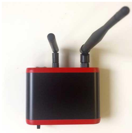
Fig. 3.6 Zolertia Orion Router, Border Router
