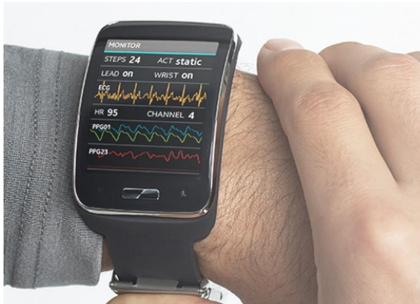
Fig. 1.4 Healthcare wearable device. The Samsung Simband™ can measure several physiological signals.
