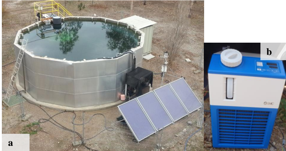
Figure 1. Solar pond pilot plant in Martorell: a) the solar thermal collectors used in the heat supply experiments and b) cooler system used in the heat extraction test.
