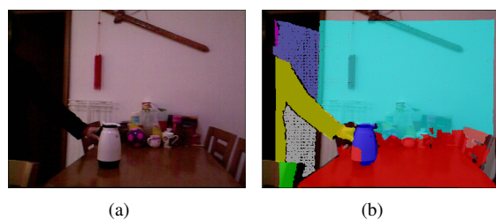
Fig. 9. An example of the segmentation result in our method: (a) a color image (b) related segmentation mask
