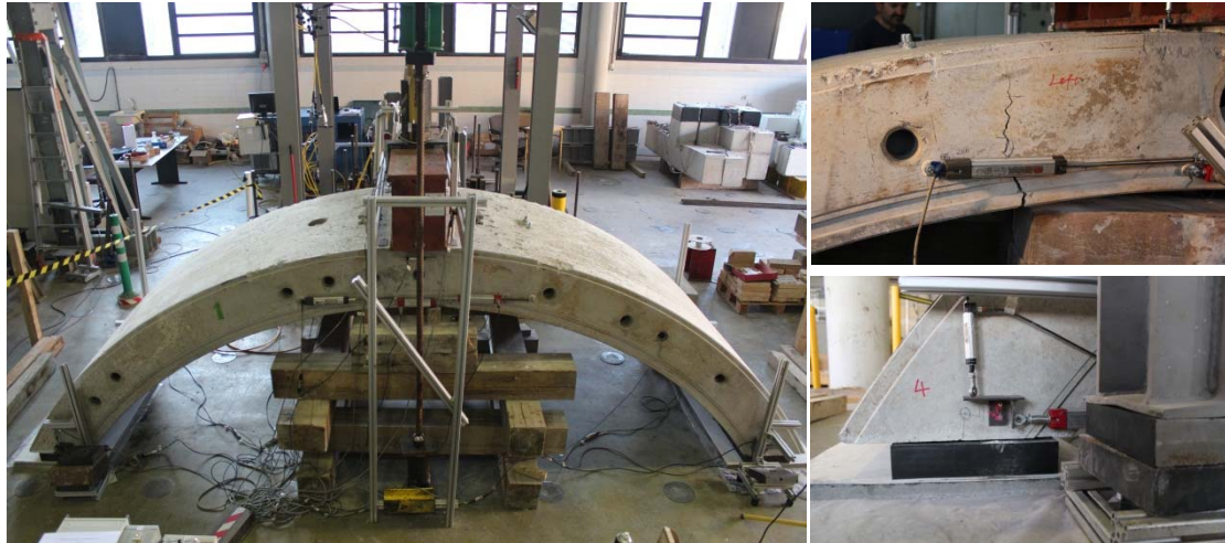
Fig. 13. (a), Segment support configuration; LVDT to measure (b) the the left face (c), roght face width of the cracks due to bending.
