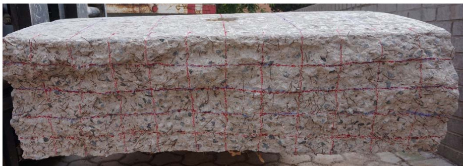
Fig. 15. Grid generated to count the fibres in the fracture sections of the segments.
