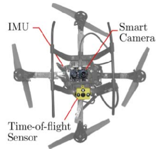
Fig.9. Bottom view of the Hummingbird quadrotor used in the experiments 9 . The vehicle is equipped with a built-in IMU, a smart camera and a time-of-flight range sensor.
