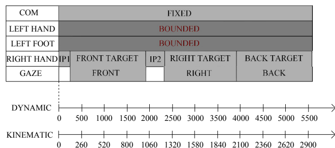
Fig. 1. Evolution of the stack of tasks designed to generate the whole-body movement of the robot.
