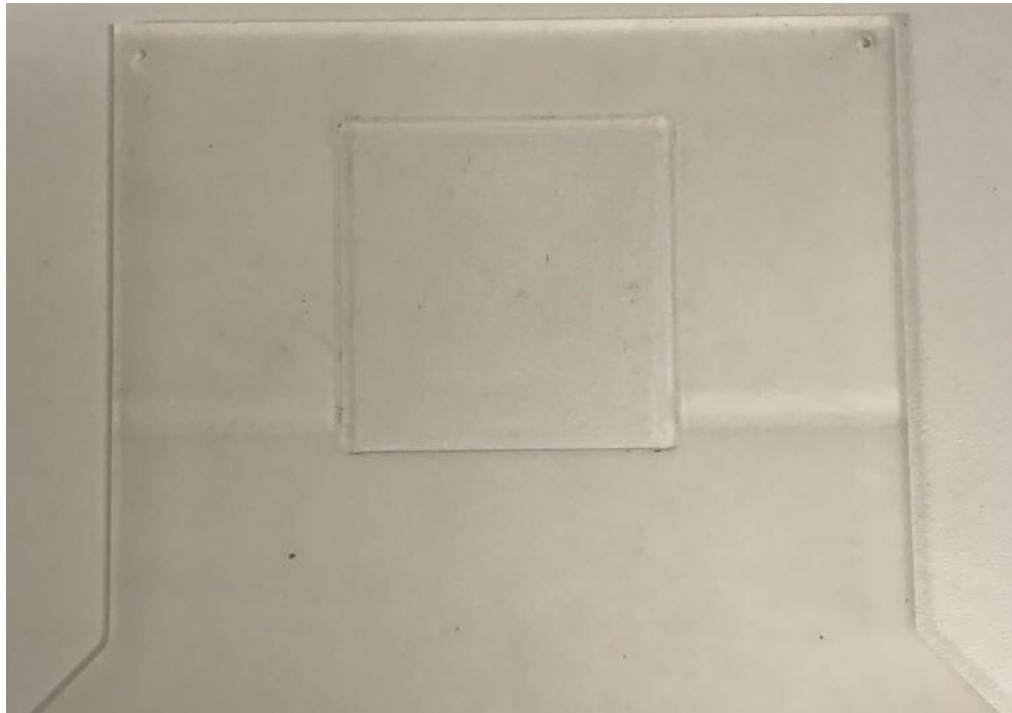
Figure 4.1: PMMA phantom to cover DUO detector with a built-in air gap
